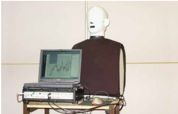
Acoustic dummy with PULSE system to measure airborne sound pressure
